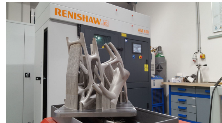
1.5.3 DMLS – Direct Metal Laser Sintering, SLM – Selective Laser Melting
